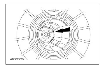
19. **NOTE:** The reverse band actuating lever must fit into the notches in the band.
